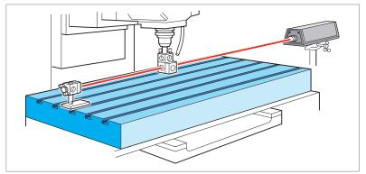
Optical setup for linear measurements
