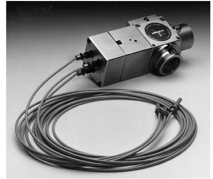
Improve positioning accuracy with more compact, lower-cost multi-axis measurements with the 10737L and 10737R compact three-axis interferometers.
